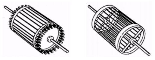
**Typical Induction Motor Rotors**
