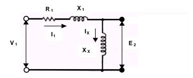
To complete the circuit, the component for the rotor equivalent must be added.
