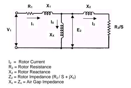
What the stator sees in the air gap is the equivalent of putting an impedance (equal to  $R_2/s + jX_2$ ) across  $E_2$ . In the analysis, all components in the motor equivalent circuit are referred to the stator.
