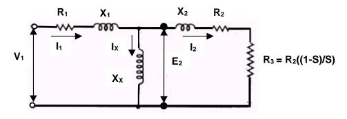
Simplifying the rotor component will yield the following per phase approximate Equivalent Circuit. This circuit will be used in the motor analysis in the sections following.
